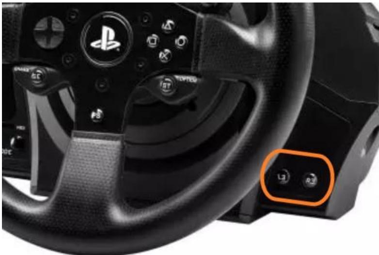
5) **Connect the T300 RS directly to a PC USB port by holding down the L3 and R3 buttons**
